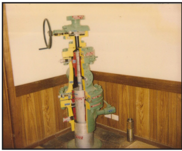
In his early days in the Australian oil patch Rick designed this model so he could teach engineers the inner workings of a gas wellhead. It is still in use today.
